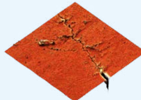
Crack propagation in metallic sample
