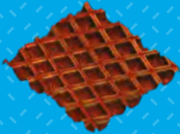
The result of anisotropic wet etching of silicon through line-grid mask, CPEM
